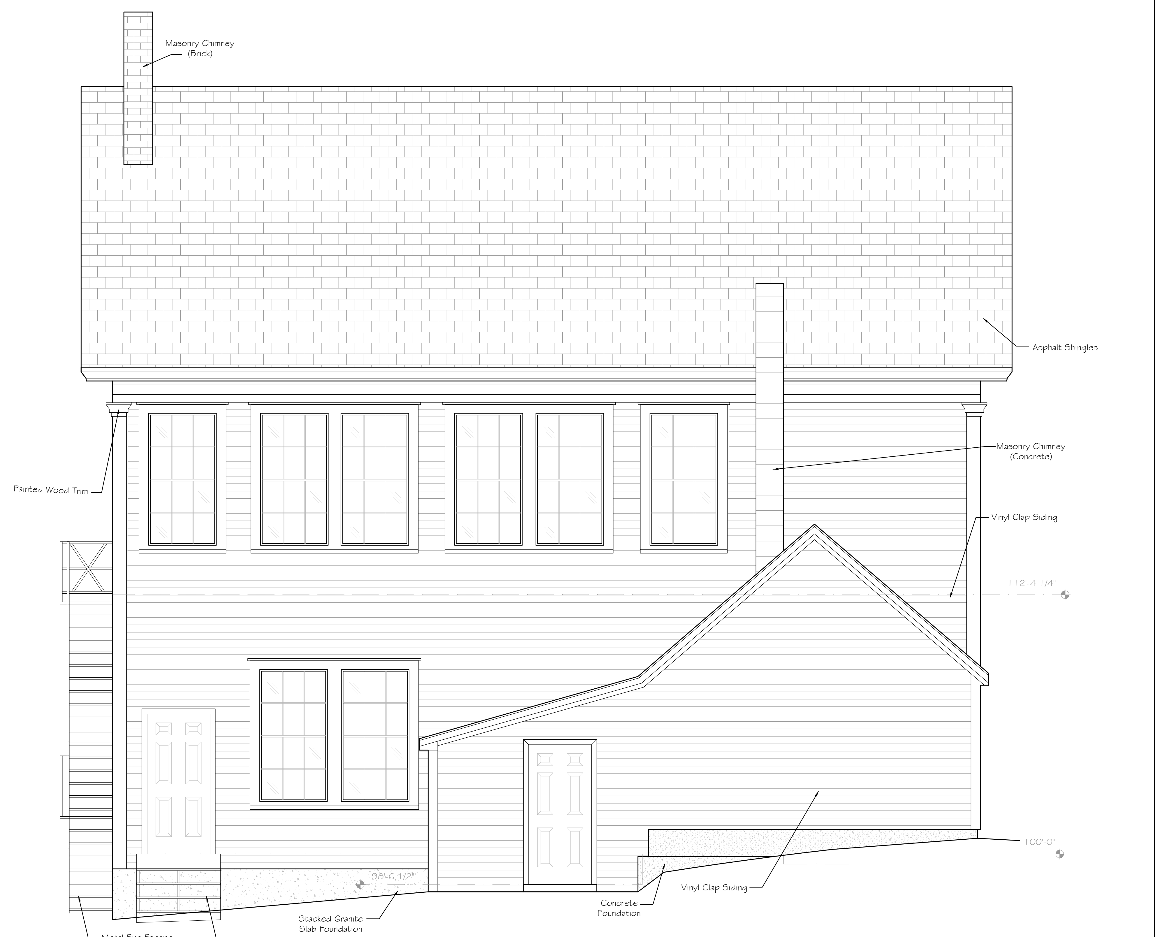
E2 NORTH ELEVATION A2.2 SCALE: 3/8" = 1'-0"
